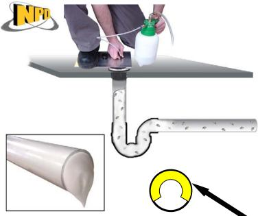
Foam can reach the organic matter that collects in areas like the top and sides of pipes and in the hollow legs of prep tables
